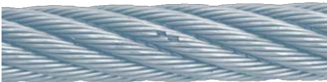
Figure 38: Condition at 40% of the bending cycle until breaking point
