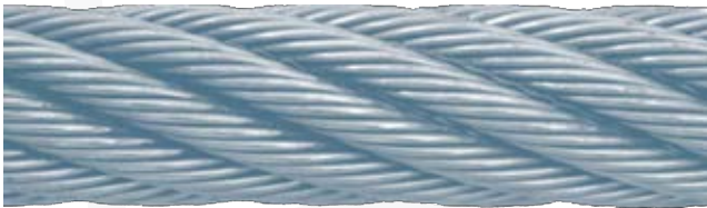
Figure 36: Condition at 0% of the bending cycle until breaking point
