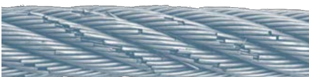
Figure 41: Condition at 100% of the bending cycle until breaking point
